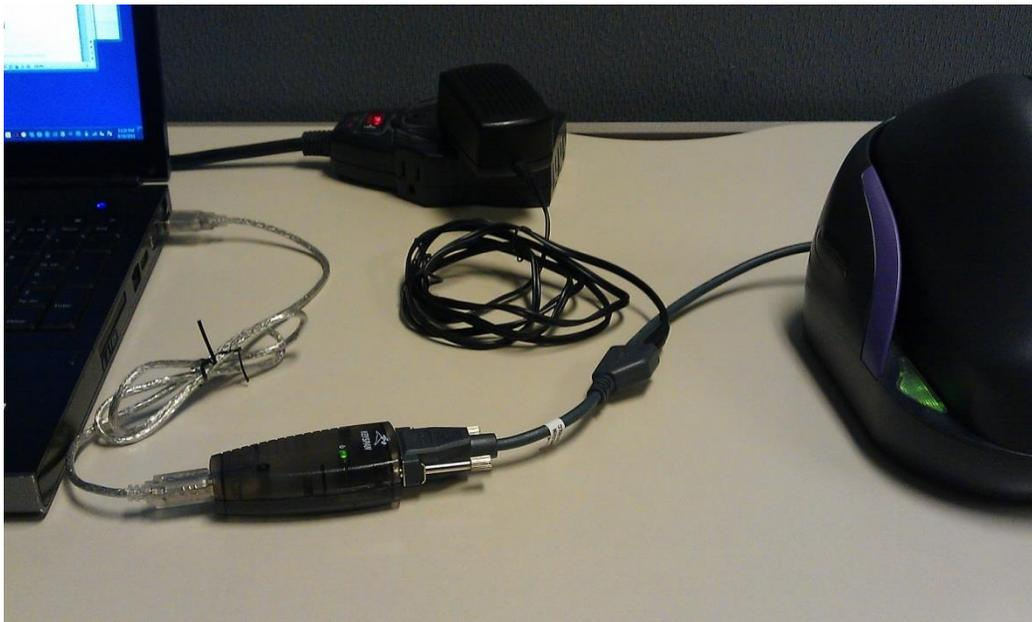
8. Lastly the Keyspan adapter USB connection will be plugged into the computer.
