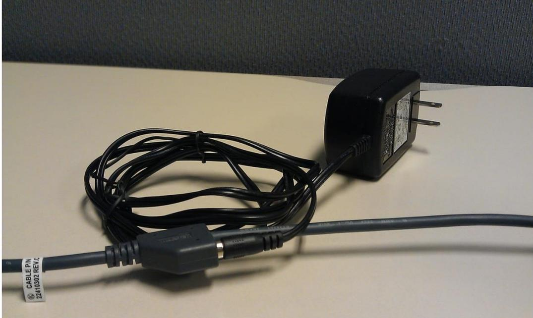
5. The power connection for the scanner is on the Magtek MICRImage Serial Cable itself.
