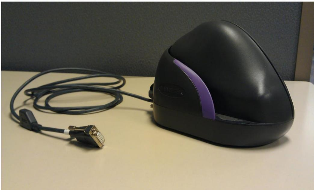
1. The Magtek Scanner and the Magtek MICRImage Serial Cable are shown here. Notice that the connector is a small square serial connector.
